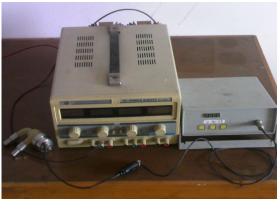
Figure1. The left ventricular assist device with impeller pump (left), direct current supply (middle) and controller (right).
